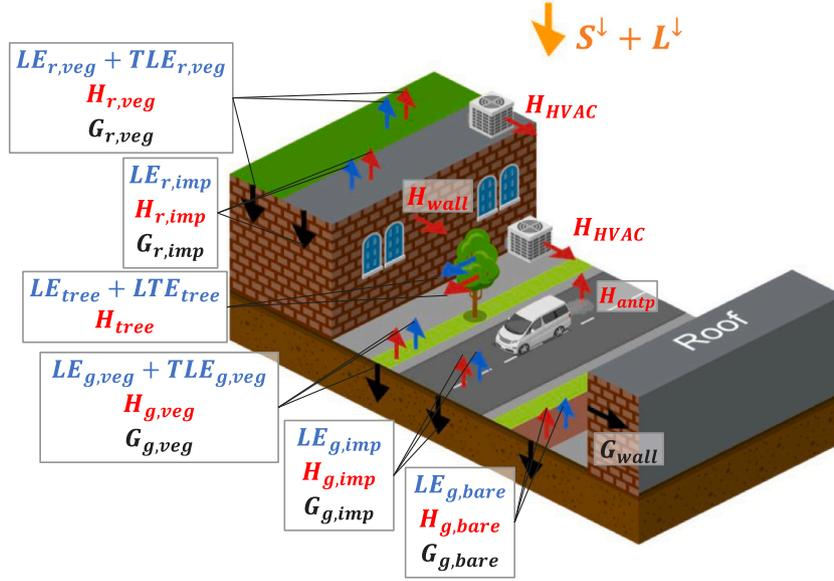
Fig. 2. Illustration of surface energy balance model in the urban area involving shortwave  $S^{\downarrow}$ , longwave  $L^{\downarrow}$ , sensible  $H$ , latent  $LE$ , evapotranspiration latent  $TLE$ , and ground  $G_i$  heat fluxes [ $W m^{-2}$ ].
