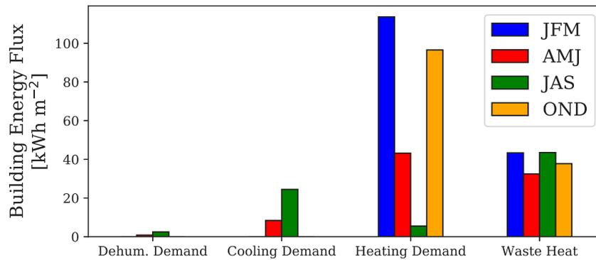
Fig. 7. Seasonal variation of the total building energy fluxes integrated over a three-month period including cooling demand ( $Q_{cool}$ ), dehumidification demand ( $Q_{dehum}$ ), heating demand ( $Q_{heat}$ ), and building waste heat ( $Q_{waste}$ ) within JFM (January, February, and March), AMJ (April, May, and June), JAS (July, August, and September), and OND (October, November, and December) months. The simulation is conducted for Vancouver in 2007.
