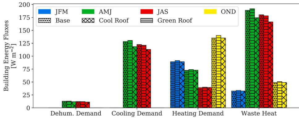
Fig. 12. Effects of green and cool roofs on building energy performance in different seasons; the building energy fluxes are mean of daily maximum over January–February–March (JFM), April–May–June (AMJ), July–August–September (JAS), and October–November–December (OND) in Vancouver 2007. (For interpretation of the references to color in this figure legend, the reader is referred to the web version of this article.)
